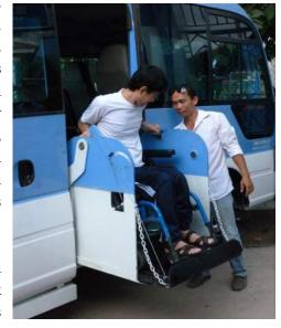
injuries. The solution is to create a lift capable of lifting both the wheelchair and its occupant, up, in, out, and off the bus. No such lift exists commercially in Viet Nam; no such bus equipped that way either, so we had one custom built by a machine shop. The sight was wonderful when the newly refitted bus, sky blue in color, arrived at the Take Wing Center to test its new lift on its handicapped family members.
